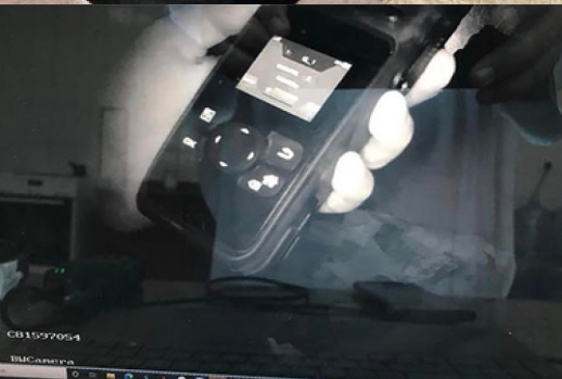
Live video screenshot from inside the sealed tunnel, using: 2.5MHz bandwidth, 4.9GHz frequency, 500mW RF output, antenna gain 1dBi
